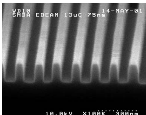
Fig. 105 High resolution images (75 nm line/space) printed in KRS by EPL (courtesy of D.M. Medeiros, IBM)
